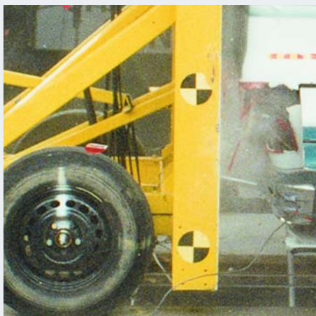
These 2 photos show the rear impact test on the 200 Chevrolet. The test vehicle was impacted by a moving barrier at 30-mph (48 km/h). The entire fuel system was then inspected for leakage. Our test vehicle did not leak any fuel.
